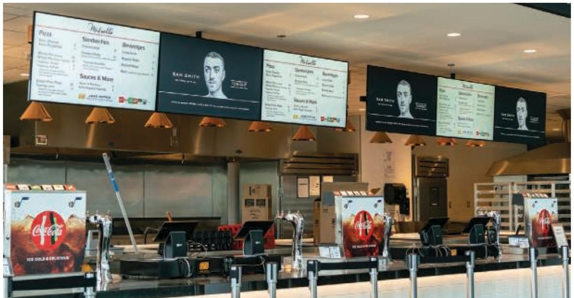
inches to 82 inches—with the majority of them being the 65-inch QM65H model; all of them have an integrated SoC player. The displays are mounted using a variety of mounts from SnapAV, Crimson AV and Solid Mounts. Fitzpatrick said the variety of applications—from menu boards to retail—dictated the need for many types of mounts.
